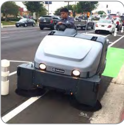
The City of Los Angeles purchases small street sweepers specifically for cycle track maintenance to ensure the facilities are clear of debris.
